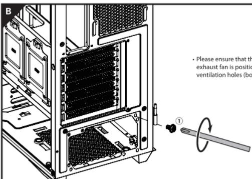
• Please ensure that the PSU intake or exhaust fan is positioned towards the ventilation holes (bottom) of the case.
