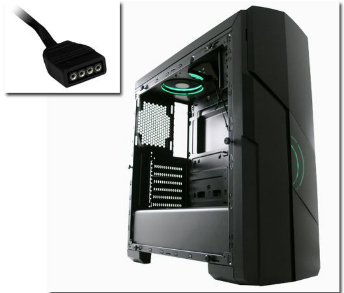
- incl. two 120 mm RGB case fans (4 pin RGB connector)
