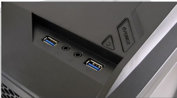
- I/O-Panel with: 2x USB 3.0 port, HD Audio
