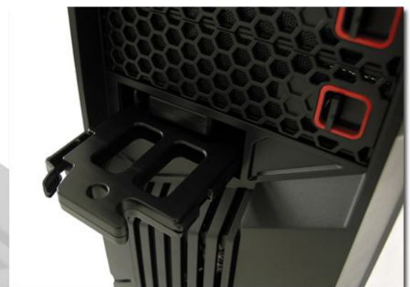
- hot swap feature for two external 2,5" HDDs/SSDs
