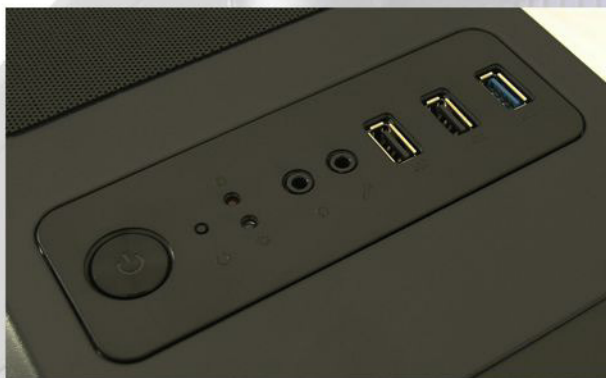
- I/O-Panel with: 1x USB 3.0 port, 2x USB 2.0 port, HD Audio
