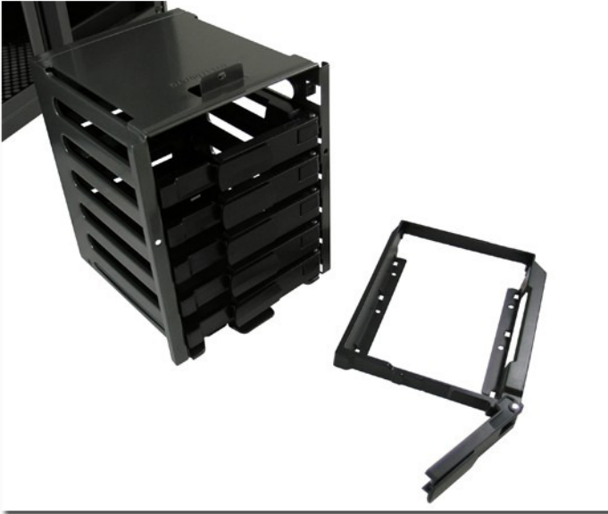
- removable mounting frame for 3,5" HDDs with hot swap feature
