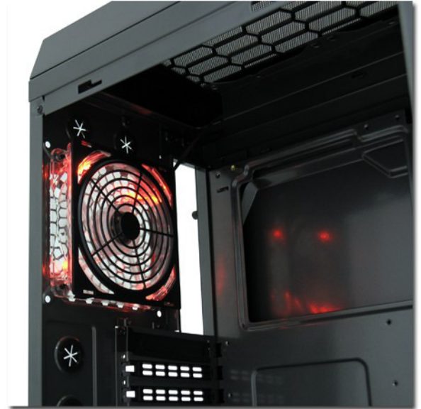
- incl. three red lighted 120 mm case fans (up to eight case fans mountable)
