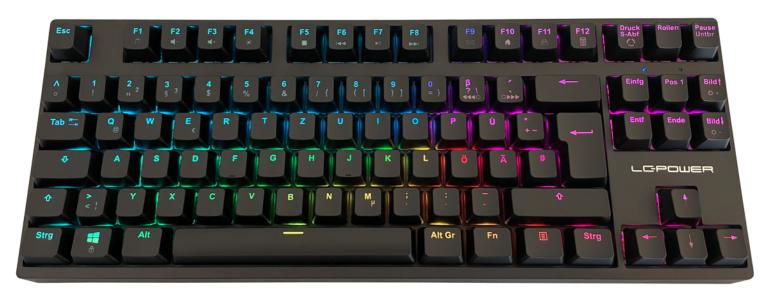
The LC-KEY-MECH-2-RGB-C-W is a compact mechanical TKL gaming keyboard which can be operated via 2,4GHz radio, Bluetooth as well as USB connection.
