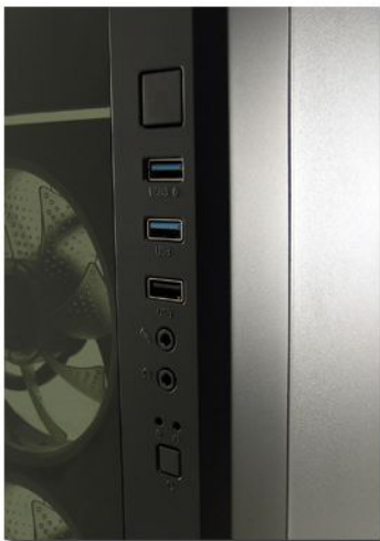
- I/O-Panel mit: 2x USB 3.0-Port, 1x USB 2.0, HD Audio
