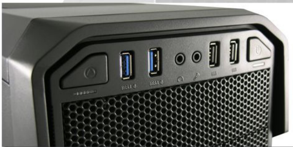
- I/O-Panel mit: 2x USB 3.0-Port, 2x USB 2.0-Port, HD Audio
