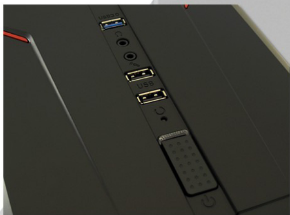
- I/O-Panel mit: 1x USB 3.0-Port, 2x USB 2.0-Port, HD Audio
