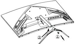
2. Push the slider next to the VESA mounting cover of the base upward (2) and tilt the stem upward (3).
