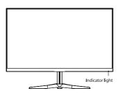
Steady blue light indicates that the power is on and the monitor works normally.
