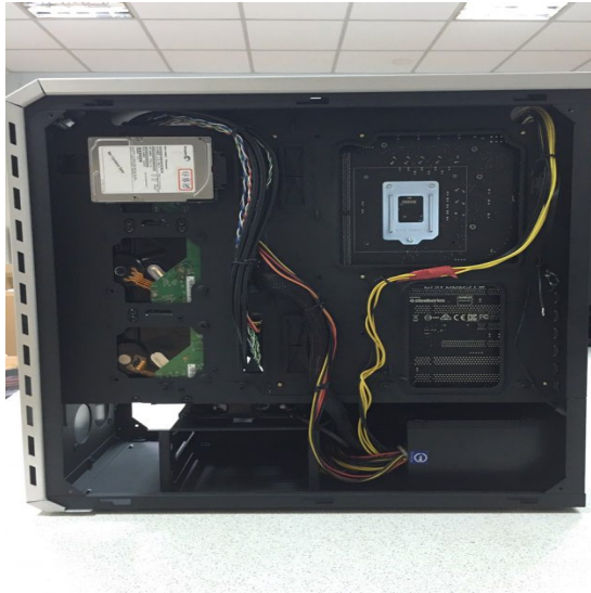
# Additional 3x 2.5" HDD/SSD on MB tray
