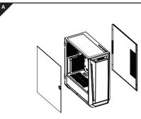
Remove front and side panel retaining screws before attempting to remove either of the panels.
