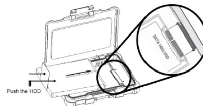
Carefully connect a 6,35cm/2,5" SATA hard disk drive (not included in delivery) with the matching connector of the PCB interface.
